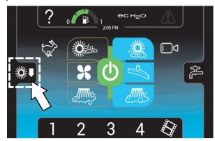
Use the *brush pressure increase* (+) *button* and the *brush pressure decrease* (-) *button* to change the brush pressure. The *brush pressure indicator bar* displays the current brush pressure setting.
