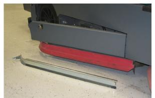
5. Remove the side squeegee blade. If the outer edge of the squeegee blade is not worn, rotate the squeegee blade with the blade from the other side of the machine. Discard the squeegee blade if both edges are worn.
