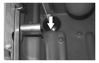
9. Close the recovery tank Variable Drain Valve.
