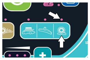
NOTE: NOTE: The scrubbing mode and the sweeping mode cannot both function at the same time. The scrubbing mode will cease operating and the sweeping mode will begin operating if any sweep button is pressed while the machine is in the scrubbing mode.
