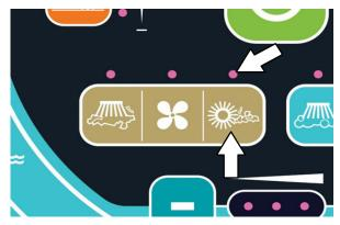
NOTE: The sweeping mode and the scrubbing mode cannot both function at the same time. The sweeping mode will cease operating and the scrubbing mode will begin operating if any scrub button is pressed while the machine is in the sweeping mode.
