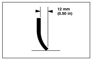
3. To adjust the overall squeegee blade deflection, turn the adjustment knobs counterclockwise to increase deflection or clockwise to decrease deflection.
