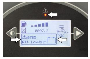
The LCD will display a fault / alert code. If there is more than one fault, each fault code will alternately display.
