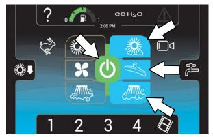
The edges of all selected sweeping and scrubbing buttons will be illuminated to show that they are in the standby mode prior to the 1-STEP button being pressed. The selected buttons will become fully illuminated when the 1-STEP button is pressed.
