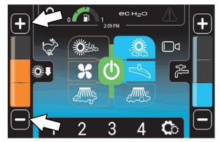
3. Use the *solution increase* (+) *button* and the *solution decrease* (-) *button* to set the zone solution flow level.
