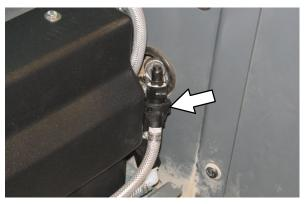
Blow pressurized air (less than 344 kPa (50 psi)) into the *ec–H2O* system outlet hose. Continue blowing compressed air into the outlet hose until water no longer drains from the drain tube
