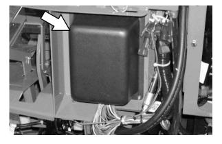
NOTE: Always replace a fuse with a fuse of the same amperage. Extra 15 Amp fuses are provided inside the relay panel drawer on the relay panel.
