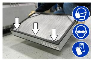
AIR–Always wear eye protection when using compressed air. Blow air through the dust filter opposite the direction of the arrows. Never use more than 690 kPa (100 psi) of air pressure and never hold the nozzle closer than 50 mm (2 in) to the filter. This may be done with the dust filter in the machine.
