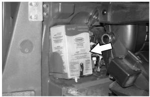
Remove the perforated knock outs from the new FaST-PAK carton. Do Not remove the bag from the carton. Pull out the hose connector located on the bottom of the bag and remove the hose cap from the connector.
