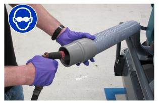
6. Rinse dirt and debris out the open drain.
