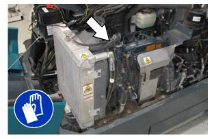
Check the radiator core exterior and hydraulic cooler fins for debris after every 100 hours of operation. Blow or rinse all dust through the grille and radiator fins, in the opposite direction of normal air flow. Be careful to not bend the cooling fins when cleaning. Clean thoroughly to prevent the fins from becoming encrusted with dust. To avoid cracking the radiator, allow the radiator and cooler fins to cool before cleaning.
