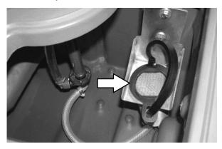
8. Rinse dirt and debris towards the recovery tank drain. Allow the recovery tank to drain.
