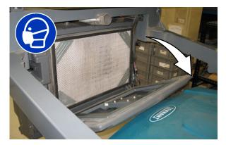
7. Remove the dust filter and perma–filter tray from the hopper.
