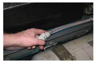
4. Pull the drain tube from the between the ec-H20 unit and the operator compartment, remove the cap from the tube, and place the end of the tube into an empty container. Set the cap aside.
