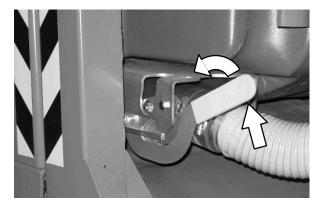
10. Reinstall the recovery tank drain hose onto the back of the recovery tank and close the recovery tank cover.
