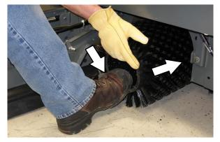
7. If rotating the brushes, always rotate the front with the back so that they wear evenly. They may be rotated end-for-end as well.
