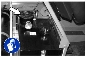
Replace the hydraulic strainer outlet after every 2400 hours of operation.
