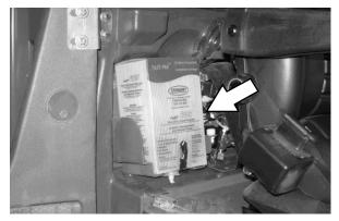
NOTE: Do not use the FaST or ec–H2O system when there are conventional cleaning detergents in the solution tank. Drain, rinse, and refill the solution tank with clear cool water before operating the FaST or ec–H2O system. Conventional cleaning detergents may cause a FaST / ec–H2O system failure.
