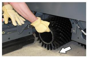
6. Install the new or rotated brushes by pushing down on the ends while sliding them onto the drive motor hubs.
