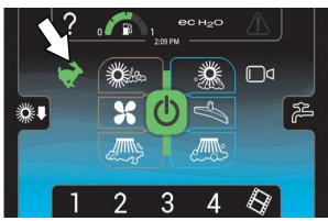
The *engine speed button* is off when the engine is in the low speed setting.
