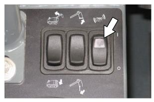
3. After the filter shaker stops, press and hold the top of the *Hopper raise/lower switch* to raise the hopper. Release the button when the hopper is at the desired position.
