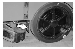
6. Route the tie-downs to the opposite ends of the machine and hook them to the brackets on the floor of the trailer or truck. Tighten the tie-down straps.
