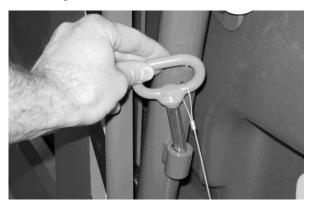
5. Insert the hopper support pin into one of the three hopper support holes. Lower the hopper until it rests on the support pin.
