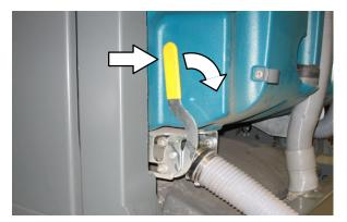
5. Remove the recovery tank drain hose from the back of the recovery tank, then rinse the dirt and debris from the hose into the tank.
