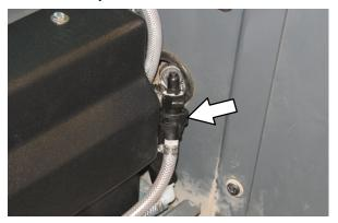
Place the *ec–H2O* system intake hose into a container containing 5 gallons (19 liters) of white or rice vinegar. Place the outlet hose into an empty bucket.
