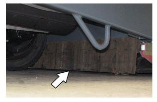
The skirts should be between 0 to 6 mm (0 to 0.25 in) from the floor when the scrub head is down.
