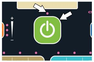
NOTE: If the machine was using the sweeping functions, the filter shaker automatically shakes the filter for a short time each time the 1–STEP button is turned off.
