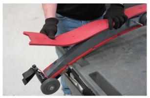
8. Install the new rear squeegee blade or rotate the existing blade to the new edge. Be sure all the holes in the squeegee blade are hooked onto the tabs.
