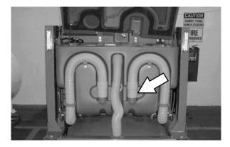
3. Open the solution tank Variable Drain Valve.
