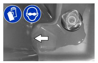
5. Rinse the float sensor and the screen filter. Allow the solution tank to drain.
