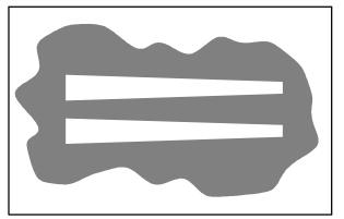
8. The brush patterns should be 50 to 75 mm (2 to 3 in) wide with the brushes in the lowered position and both patterns should be the same width. If the width of the brushes is not the same, see *ADJUSTING THE MAIN BRUSH WIDTH* section of this manual.
