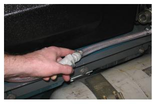
Disconnect the *ec–H2O* system outlet hose from the hose to the scrub head and connect the outlet flush hose (black connector) to the *ec–H2O* system outlet hose.
