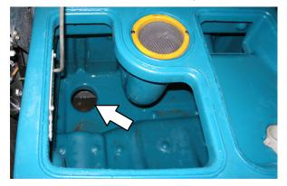
7. Clean the drain hole, then reinsert the drain plug. Push the handle down to tighten. Be sure the drain plug is fully seated before tightening.
