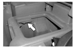
Open the recovery tank cover and fill the recovery tank with water (not to exceed 60°C / 140°F) until the recovery tank is approximately half full.
