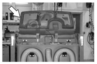
2. Place the recovery tank drain hose nozzle next to a floor drain.
