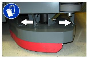
3. Open the retaining band tension latch.
