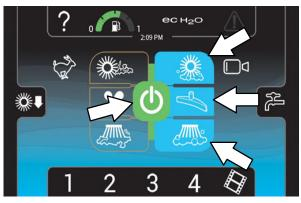
NOTE: DO NOT turn on the FaST or ec-H2O system during conventional scrubbing. Conventional cleaning detergents could cause a FaST or ec-H2O system failure. Drain, rinse, and refill the solution tank with cool clean water before operating the FaST or ec-H2O system.
