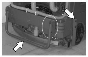
To engage the rear squeegee protector, pull the pin, lower the protector bar, and reinsert the pin.
