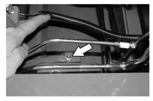
On the other side of the machine the torque tube grease fittings are located beneath the propel pump.
