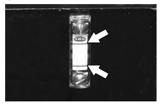
ATTENTION! Do not overfill the hydraulic fluid reservoir or operate the machine with a low level of hydraulic fluid in the reservoir. Damage to the machine hydraulic system may result.
