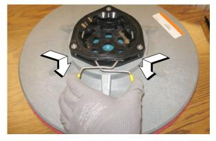
6. Place the new side brush underneath the side brush assembly and lift the side brush up onto the side brush hub until the brush locks onto the hub.
