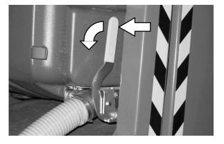
4. Rinse the solution tank. Flush dirt and debris toward the solution tank drain.
