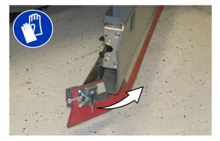
4. Remove the retaining band from the side squeegee assembly.
