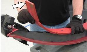
13. Install the new front squeegee blade or rotate the existing blade to the new edge. Be sure the holes in the squeegee blade are hooked onto the tabs.
