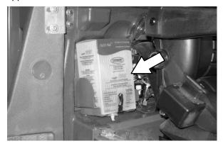
When in the optional ES (Extended Scrub) mode, the dirty solution in the recovery tank is filtered through the ES system and returned to the solution tank for reuse. Detergent is then injected into the returned solution to revitalize the cleaning capability of the solution.
