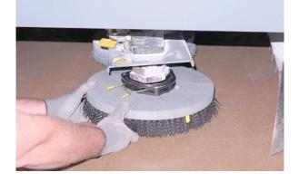
5. Set the brush spring open on the new brush to make installation easier.
