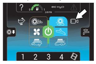
The camera automatically comes on when the bottom of the *directional pedal* is pressed to place the machine in reverse and remains on the entire time the machine is in reverse.
