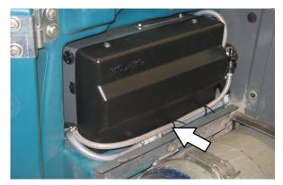
13. Return the intake flush hose to the storage bag behind the operator seat.
