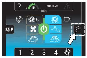
Use the *solution increase* (+) *button* and the *solution decrease* (-) *button* to set the solution fl ow level. The *solution flow indicator bar* displays the current solution flow setting.
