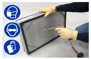
WATER–Rinse the dust filter with a low pressure garden hose through the dust filter opposite the direction of the arrows.
