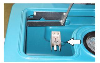
7. ES machines: Rinse the ES filter. If necessary, remove the ES filter from the recovery tank.
