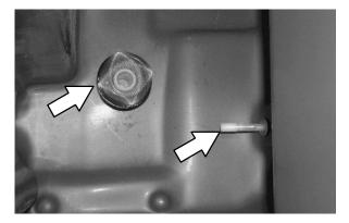
6. Close the solution tank Variable Drain Valve.
