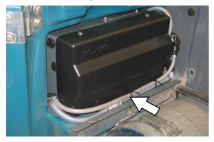
NOTE: The outlet and intake hoses must be down between the ec–H2O assembly and the bracket so they are not pinched or damaged when the operator seat cover is closed.
