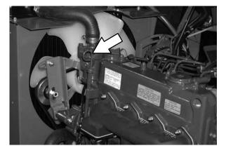
Fill the engine with oil until the oil is between the indicator marks on the dipstick. DO NOT fill past the top indicator mark. The engine oil capacity is 6 L (6.35 qt) with oil filter.
