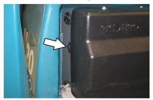
NOTE: The module will automatically shut off when the flush cycle is complete (approx. 7 minutes). The module must run the full 7 minute cycle in order to reset the system indicator light and alarm.
