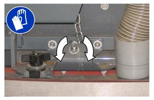
4. Turn the squeegee leveling nut counter-clockwise to decrease the deflection at the ends of the squeegee blade.
