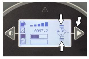
When two thicker bars appear above and below the engine speed icon and the thinner bars and the icon is solid the engine is in the high setting.
