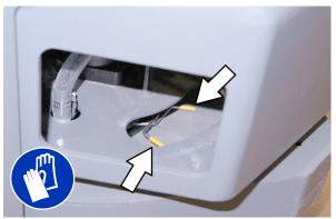
4. Remove the side brush from underneath the side brush assembly.
