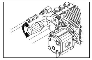
NOTE: Adjust the pressure at the wand before adjusting it at the system.
