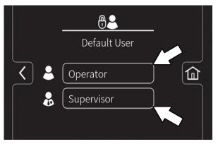
5. Select a pre-assigned user profile. Turn off the machine to apply the setting.
