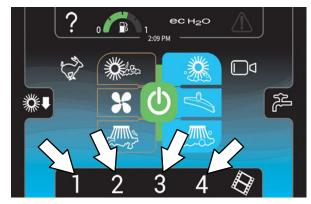
Press the required zone control button. The selected preset button will illuminate and the name of the zone appears above the button. The *solution flow indicator bar* / adjustment buttons and *brush pressure indicator bar* / adjustment buttons briefly appear in the display to show the settings for the selected zone.
