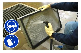
NOTE: If water is used to clean the dust filter, be sure the filter is completely dry before reinstalling it into the hopper. **<u>Do Not</u>** reinstall a wet dust filter.
