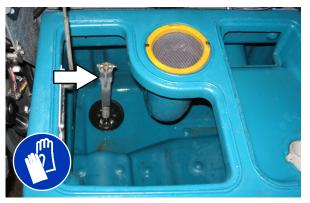
4. Open the recovery tank Variable Drain Valve.
