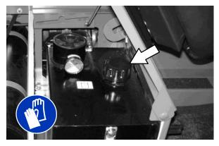
Replace the hydraulic fluid filter after every 1200 hours of operation or if the hydraulic reservoir gauge is in the yellow/red zone when the reservoir hydraulic fluid is approximately  $32^{\circ}$  C ( $90^{\circ}$  F).
