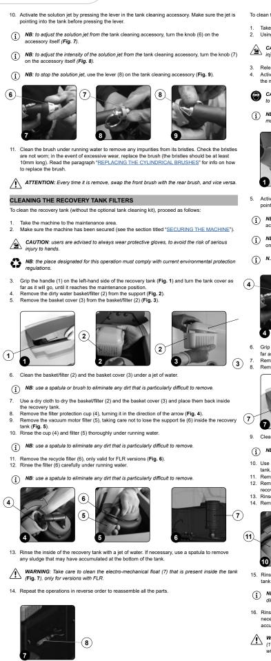
To clean the recovery tank filters (with the optional spray gun kit), proceed as follows:
