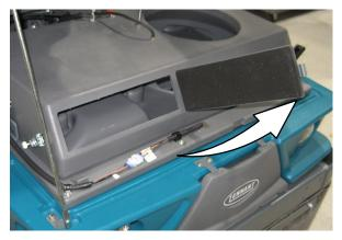
3. HEPA Machines: Use a HEPA certified vacuum to clean dust and debris from the interior of the upper cyclone chamber.
