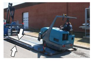
3. To winch the machine onto the truck or trailer, attach the winching chains to the rear tie down locations. The rear tie-down locations are the holes in the sides of the machine frame near the rear bumper.  Turn the bypass valve 90° from the normal position before winching the machine onto the truck or trailer. See *PUSHING OR TOWING THE MACHINE* section of this manual. Make sure the machine is centered.
