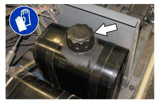
Machines (S/N 005694- ) have a fluid level gauge on the hydraulic tank. The hydraulic fluid level should be between the two lines on the hydraulic gauge.
