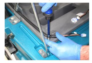
9. Remove the four brackets securing the lower cyclone chamber to the hopper.
