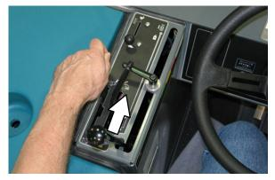
11. Push the hopper door lever forward to open the hopper door.
