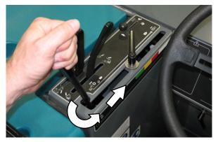
6. Place the side brush lever in the left **Side brush down and on** position. The brush will automatically start rotating.
