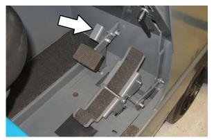
FOR SAFETY: When starting machine, keep foot on brake and directional pedal in neutral.
