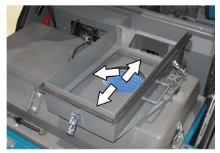
6. Reinstall the HEPA filter into the HEPA filter assembly. Be sure the arrow on the HEPA filter label is pointing up.
