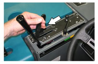
4. Shake the dust filter by holding the vacuum and filter shaker lever in the **Filter shaker** position for 30 seconds.
