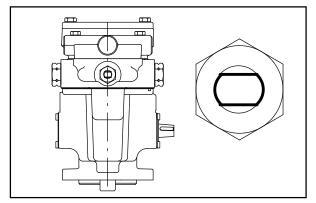
Return the bypass valve to the normal position when through pushing or towing the machine.
