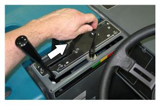
8. Pull and hold the hopper door lever back until the hopper door closed light comes on.
