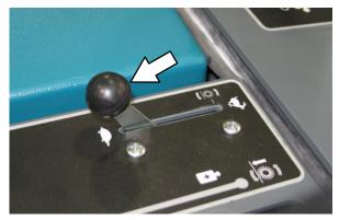
On gasoline powered machines, pull out the choke knob when the engine is cold. Push in the choke knob after the engine is running smoothly.
