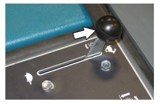
4. Pull and hold the hopper raise / lower lever back and raise the hopper to the desired height. Release the lever into the **Hold** position.
