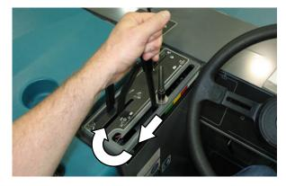
3. Pull and hold the hopper door lever back until the hopper door closed light comes on.
