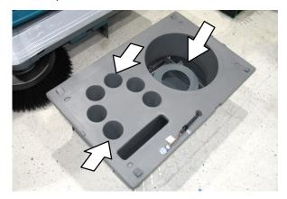
15.Inspect cyclone Perma–Filter inside the lower cyclone compartment for debris.
