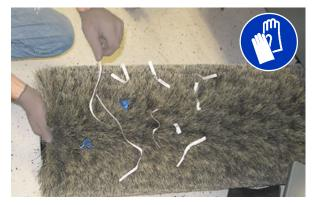
Check the main brush pattern and rotate the brush end-for-end after every 50 hours of operation, for maximum brush life and best sweeping performance. Refer to *REPLACING OR ROTATING THE MAIN BRUSH*.
