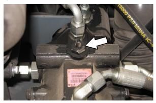
ATTENTION! Do not push or tow machine for a long distance and without using the bypass valve, or the machine hydraulic system may be damaged.
