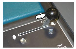
3. Pull and hold the hopper raise / lower lever back and raise the hopper slightly. Release the lever into the **Hold** position.
