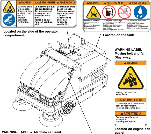
WARNING LABEL – Machine can emit excessive noise. Hearing loss can result. Wear hearing protection.
