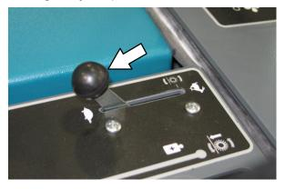
8. Shut the machine off.
