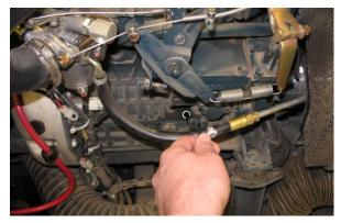
Fill the engine with oil until the oil is between the indicator marks on the dipstick. DO NOT fill past the top indicator mark. The engine oil capacity is 3.4 L (3.6 qt) with oil filter.
