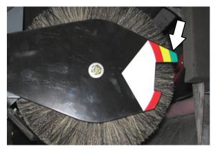
2. Loosen the main brush adjustment knob and slide the knob so it matches the color band on the brush idler plate. Retighten the knob.
