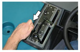
FOR SAFETY: When using machine, do not raise hopper when machine is on an incline. Make sure adequate clearance is available before raising hopper.
