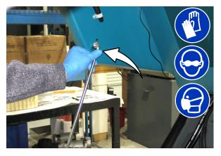
2. Loosen the three clamps securing the cover to the HEPA filter assembly and remove the cover.
