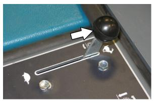
9. Release the machine parking brake.
