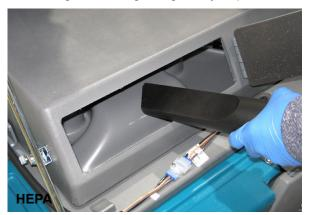
4. HEPA Machines: Use a HEPA certified vacuum to clean the slots located at the top of the dust filter compartment.
