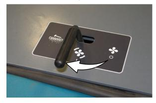
NOTE: The vacuum fan duct should be off when sweeping wet debris.
