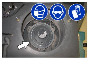
2. Machines (S/N 006266- ), open the front clean out door on the upper cyclone chamber and clean.
