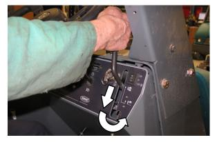
2. Place the main brush lever in the left **Main brush up and off** position.
