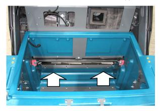
14.Use a garden hose to clean out the filter compartment and lower cyclone compartment.
