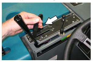
11. Move the vacuum and filter shaker lever into the **Vacuum fan on** position.
