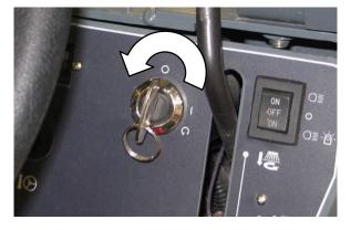
FOR SAFETY: Before leaving or servicing machine, do not park near combustible materials, dust, gases, or liquids. Stop on level surface, set parking brake, turn off machine, and remove key.
