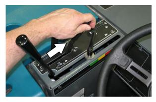
12. Move the vacuum and filter shaker lever into the **Vacuum fan on** position.
