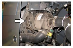
To remove the filter element, raise the hopper and engage the hopper support bar. Set the parking brake and turn the engine off. Remove the top two dust skirt clips and pull back the dust skirt to access the air filter housing.
