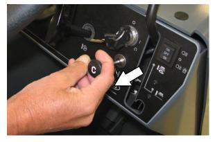
5. Turn the ignition switch key clockwise until the engine starts.
