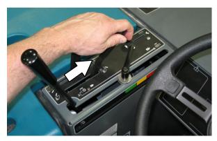
4. Move the vacuum and filter shaker lever to the **Vacuum fan on** position.
