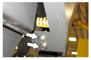
The side brush front to rear tilt is adjusted with the side brush cable and clevis pin.
