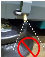
To adjust the spray pattern, use the water valve located next to the the water tank. Do not open the valve to the 90° maximum position. Optimal position is with the valve opened between  $10-15^{\circ}$
