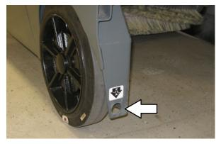
The rear tie-down locations are the holes in the sides of the machine frame near the rear bumper.
