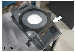
Use both hands to firmly grasp the dust filter and carefully lift the dust filter from the dust filter compartment. <u>DO NOT</u> use the seal to lift the dust filter from the dust filter compartment.
