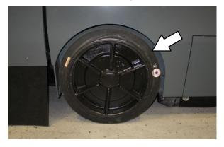
Check the front tires after every 100 hours of operation for damage. Check the rear tire pressure after every 100 hours of operation. The proper tire pressure is 795 kPa (115 psi).
