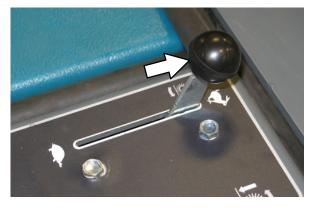
3. Push the hopper door lever forward to open the hopper door.
