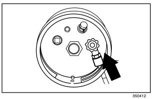
9. Open the tank service valve slowly and check for leaks. Close the service valve immediately if an LPG leak is found, and tell the appropriate personnel.
