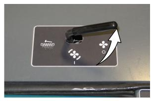
NOTE: Excessive heat in the hopper will cause the Thermo Sentry to move the vacuum and filter shaker lever to the **Vacuum fan off** position. It will also make the hopper temperature light come on. If this happens, stop the machine, eliminate the source of the heat, and return the lever to the **Vacuum fan on** position.
