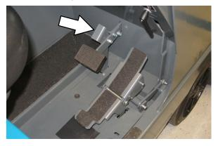
NOTE: If the operator is not in the seat, the parking brake must be engaged or the machine will automatically shut off after 2 seconds.
