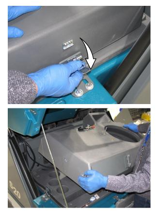
5. Inspect and clean the upper cyclone chamber seal. Replace seals if they are damaged or worn.
