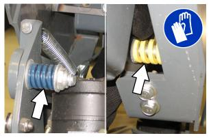
The side brush side tilt (left to right) is adjusted with the two bolts.
