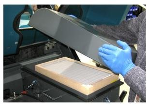
3. Remove the HEPA filter from the HEPA filter compartment.
