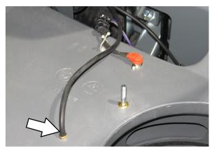
2. Disconnect the main wire harness from the filter shaker assembly and remove the filter shaker assembly from the filter compartment.
